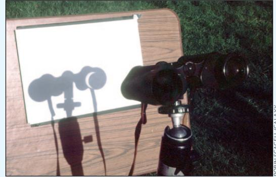
Sun drifts out of the field of view, it might melt the inside of the eyepiece! So take great care, or use an old eyepiece (many older eyepieces used metal rather than plastic).
